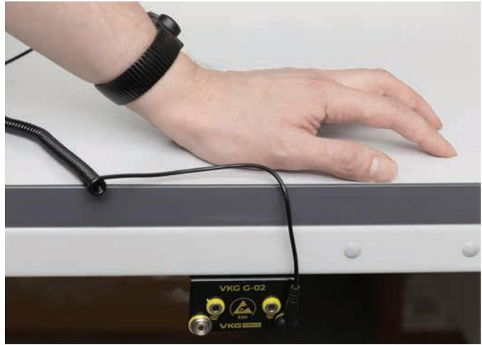
The ESD wrist straps are used to electrically connect, or bond people and other conductors to ground, to create an equipotential balance between all items and people within the ESD Protected Area (EPA). The fully adjustable wrist straps with conductive fibers are comfortable and hypoallergenic. They must be complemented with wrist strap ground ((EPA)VKG A-3146 Grounding unit) or banana plugs.
