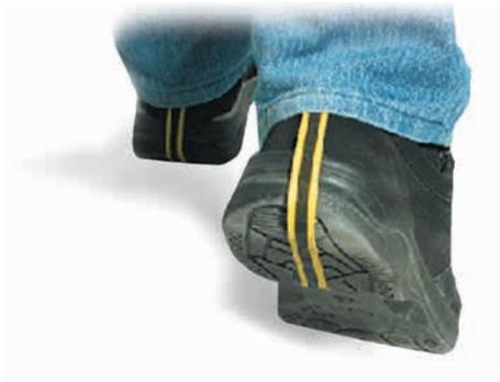
These disposable ESD heel straps are specially designed to provide a continuous ground path between the user and a properly grounded ESD floor or floor matting material. Easy deployment, secure attachment to all shoes. Simply peel liner from bottom of the strap, place adhesive strip on heel, wrap the strap up and inside of shoe and get to work!
